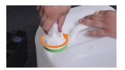
Close the old cartridge with a sealing cap and hand-tighten it with the barrel wrench by turning it clockwise.
