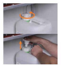
Remove the dispensing head of the Ecoport or the multi tank connector from the connected cartridge by turning it counterclockwise.
