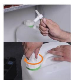
Open the cap of the full cartridge using the barrel wrench (this is included in the accessories of your Ecoport) by turning it counterclockwise
